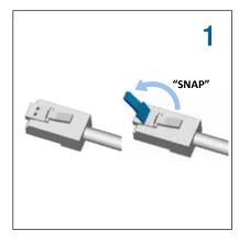
Snap or cut off release tab of the RJ45 plug.
