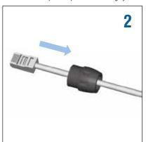
Slide the nut (backshell) onto the cable.
