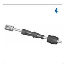
Close clamp-boot, fasten the two tabs together to lock.
