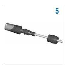
Push clamp-boot & cable together into the shell
