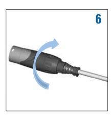
Thread the nut (backshell) onto the shell (torque 0.8Nm-1.2Nm) to close the connector assembly.
