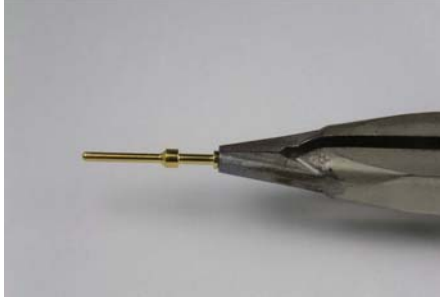
Figure 4: MP-INS-16 Insertion Pliers for Size 16 contacts
