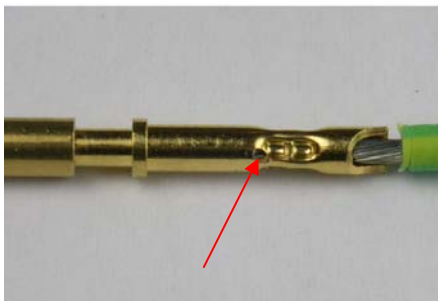
Figure 1: Good crimp – wires visible in inspection hole
