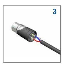
Push back the insert only enough to expose the solder buckets. It is not necessary to remove the insert. Solder the wires to the contacts.
