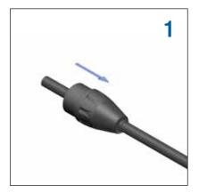
Slide the nut (Backshell) onto the cable
