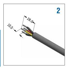
Strip the cable and twist the conductors.
