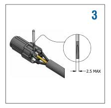
Insert the conductors into the rear of contacts on the insert. Tighten the screws to 0.35Nm (3.0 lb-in) using a flat screwdriver with tip width of 2.5mm max.
