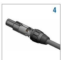
Install the cable clamp, flush to the insert making sure to align the slot as shown in the picture.
