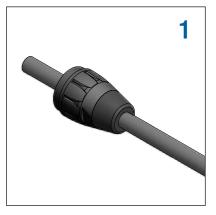
Slide the nut onto the cable
