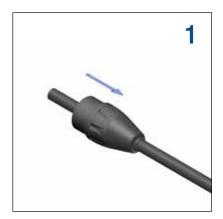
Slide the nut (Backshell) onto the cable
