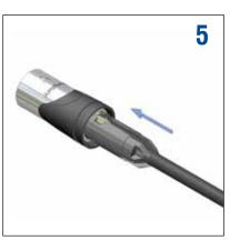
Align the key of the insert with the keyway on the shell then push the pin insert & cable clamp together in the shell.
